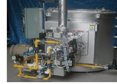
Regenerative Burners in industries, Toyotsu Machinery, Indonesia
